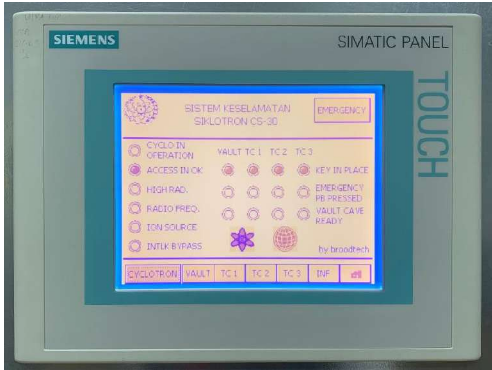
FIGURE 4. The LCD touchscreen for the safety system interface.
